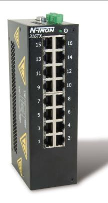
The 316TX-N switch has extended operating specifications to meet the harsh needs of the industrial environment, including extended temperature rating, extended shock and vibration specs, redundant power inputs, and a high MTBF (greater than 2M hours).
