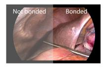
FSN's optical bonding process (right) improves contrast ratio and brightness, and increases humidity resistance and breakage resistance.
