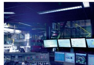
Hot Dip Galvanizing Plant 2 at Thyssenkrupp Steel Europe was modernized with a new control system. Based on a SIMATIC IPC and using the SIMATIC WinCC SCADA system, the SIMATIC Process Historian, and SIMATIC Thin Clients for visualization in the plant, the Siemens Solution Partner designed an innovative and future-oriented solution characterized by high availability and data security, thus improving the performance and process safety of the entire plant.
